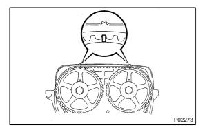
(b) Check that the timing marks of the camshaft timing pulleys are aligned with the timing marks of the No.4 timing belt cover.
