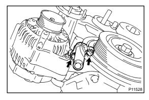
(a) Alternately loosen the 2 bolts, and remove them, the tensioner and dust boot.
