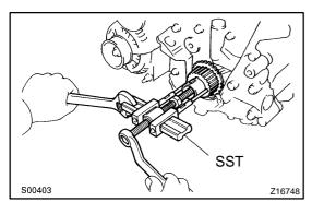
(b) Remove the crankshaft timing pulley.
