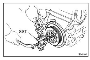
(c) Using SST, remove the pulley.
