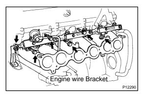
11. INSTALL INTAKE MANIFOLD AND DELIVERY PIPE ASSEMBLY
