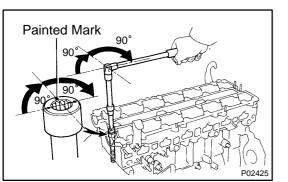
(d) Mark the front of the cylinder head bolt head with paint.
