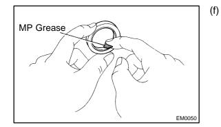
Apply MP grease to a new camshaft oil seal lip.
