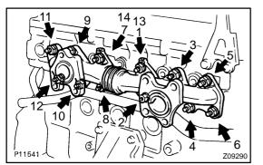
(b) Install the exhaust manifold with 12 new nuts, in several passes, in the sequence shown.
