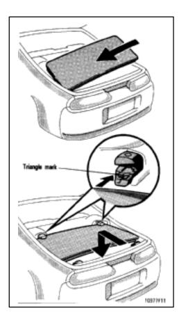
Put in the roof from the left side as shown. Then insert the front edge of the roof in the front holders, and engage the rear edge with the rear holders.
