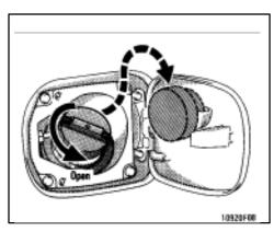
To remove the fuel tank cap, turn the cap slowly counterclockwise, then pause slightly before removing it. After removing the cap, hang it on the cap hanger.
