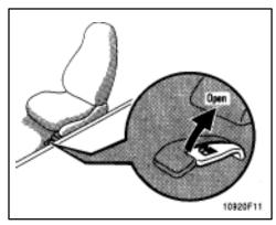
To open the fuel filler door, pull the lever up.
