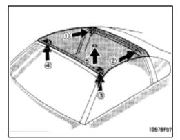
Tighten the bolts and lock the center lock in the order shown. (See "-Detaching from vehicle" for details.)
