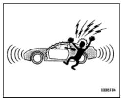
To deter the vehicle theft, the system is designed to give an alarm and keep the engine from being started if any of the side doors, back door or hood is forcibly unlocked or the battery terminal is disconnected and then reconnected when the vehicle is locked.
