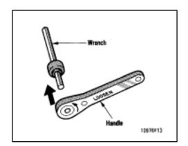
2. Face the "LOOSEN" side of the handle toward you and insert the wrench into the handle.
