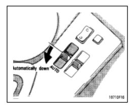
Automatic operation (to open only): Pull the switch completely down and then release it. The window will fully open.To stop the window partway, lightly push the switch up and then release it.
