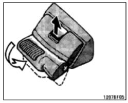
After removing the roof, put back the rear holders by pulling up the lock release knob.
