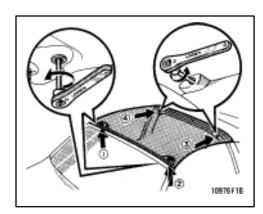
Loosen the bolts in the order shown by turning the wrench counterclockwise. Then lift up the front edge of the sport roof and lift off the roof forward.
