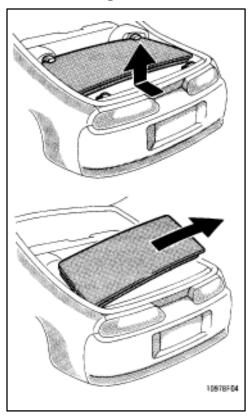
Lift up the rear edge while pushing the roof fully fowward, then pull the front edge out of the holders. Remove the roof from the right side as shown.
