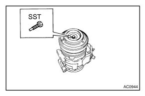
(b) Install SST on the pressure palate. SST 07112–66040
