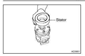
(c) Remove the stator.
